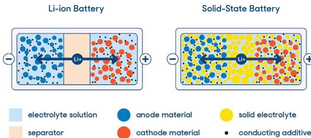
**Solid-state battery:** Like lithium-ion batteries, solid-state batteries store energy; however, instead of an organic liquid electrolyte solution sandwiched between the cathodes and anodes, solid-state batteries use solid electrolytes. Some manufacturers are planning to roll them out as early as 2027. Solid-state batteries offer higher energy density, greatly extended range and faster charging times.
