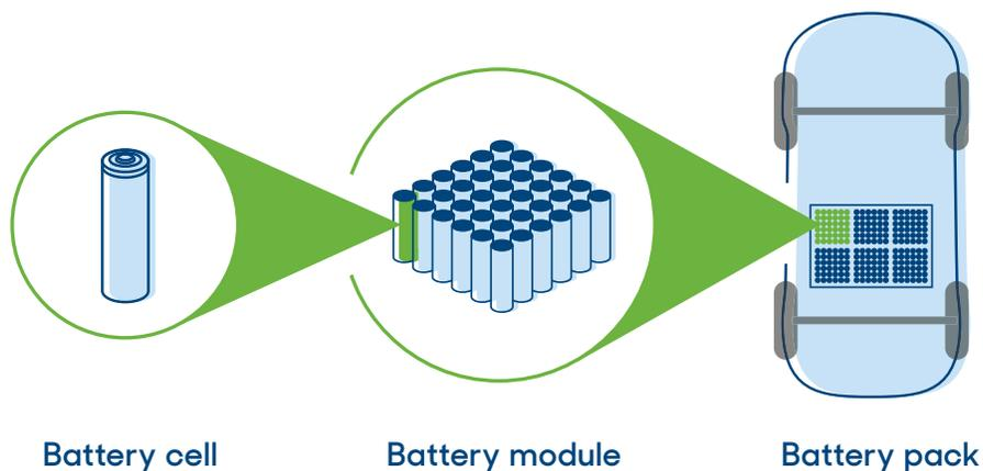
**Battery pack:** A group of battery modules. An EV's battery is where the electricity that powers your car is stored. Think of it as the fuel in your EV's "tank."
