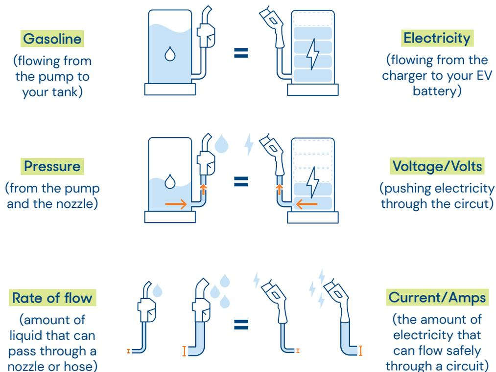
**Amps (A):** Also known as amperes, an amp is a unit of measure for electrical current flow. An EV's amp rating (or the charging station's amp rating) is one factor that determines the maximum amount of power that can be delivered to your car's battery. If **voltage** is to electricity as pressure at the gas pump is to gasoline, then **amps x volts = watts** all work together to measure how quickly you can fill up your battery with power.
