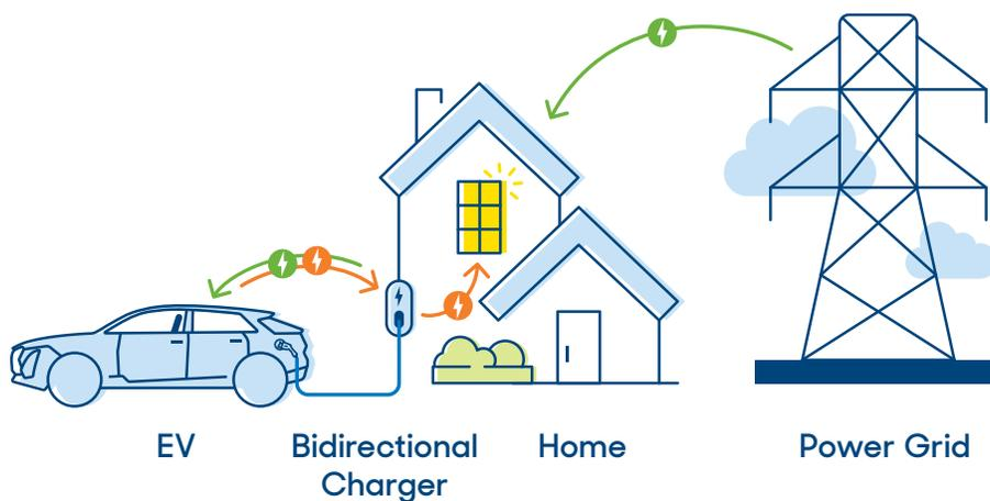
**Bidirectional charging:** A technology that allows energy to flow two ways: from the electricity grid to your EV, and from your bidirectional EV charger to the grid. See **vehicle to grid (V2G)** (future state) and **vehicle to home (V2H)** (select EVs and charger stations).
